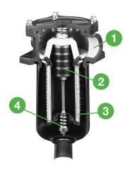
BGT Filters feature Parker's exclusive Magnetic Prefiltration core which collects ferromagnetic particles from fluid upstream of the filter element. This feature alone could save hundreds of dollars a year by protecting costly equipment from increased wear and malfunction by assuring that the fluid is as pure as possible when it leaves the filter. Even during bypass due to cold start up, ferris contaminant is collected by the magnetic core, a feature of importance on any fluid power system.
